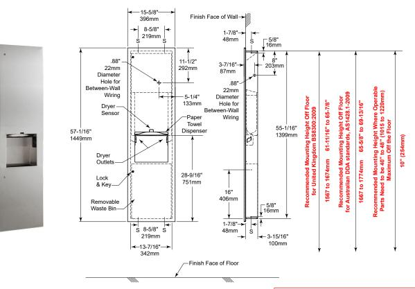
Rough Wall Opening 362mm (14-1/4") wide 1412mm (55-9/16") high 100mm (4") minimum recessed depth
