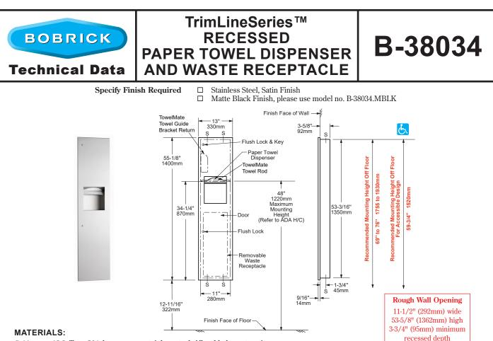
Cabinet — 18-8, Type-304, heavy-gauge stainless steel. All-welded construction.
